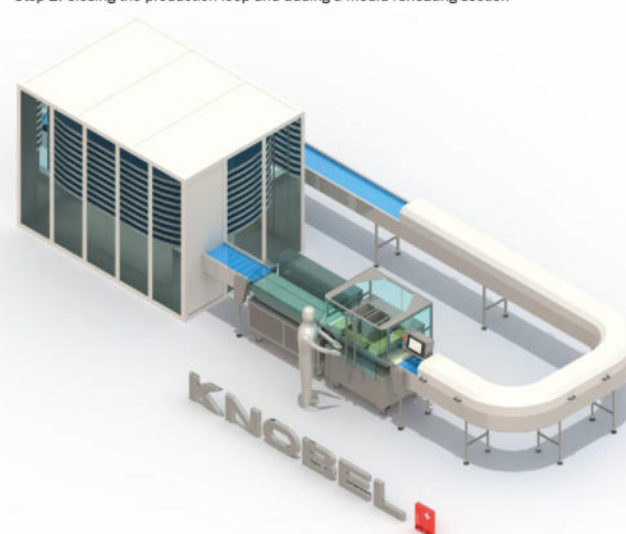
Step 2: Closing the production loop and adding a mould-reheating section
