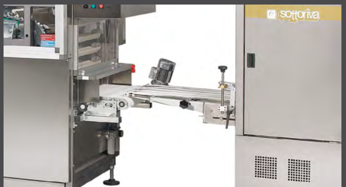
An adjustable infeed belt of the proofer allows a better control of the input pieces according with the weight and size.
