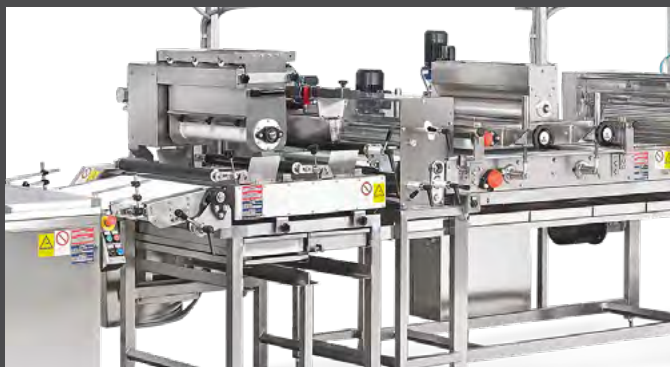
Aligner for finger roll / Hot Dogs for a straight product deposit on tray.
