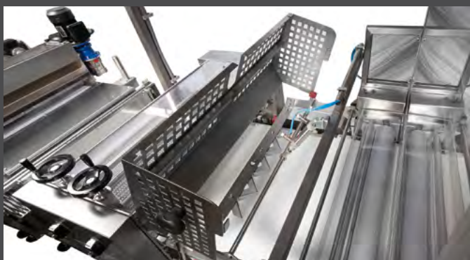
Aligner device for round products for a perfect alignment into a tray.
